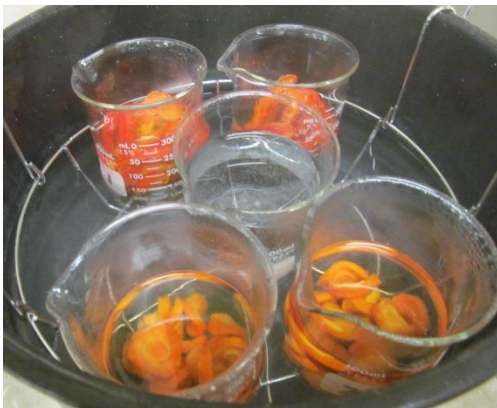
Figure 12-5: Rehydrating samples in a hot water bath
