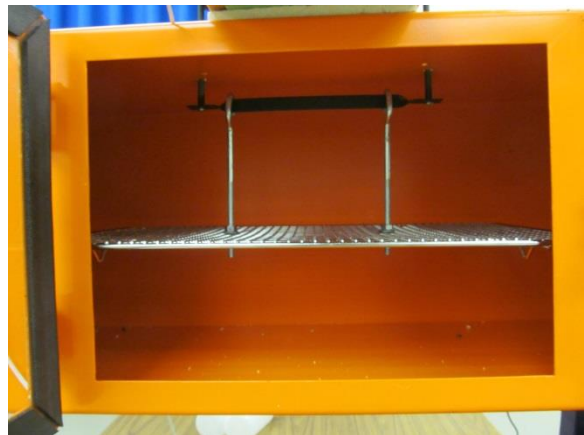
Figure 6-2: Rack inside tray dryer linked to balance on top of dryer
